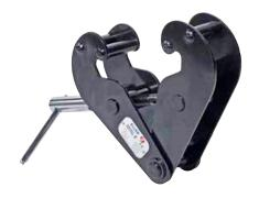
A beam clamp is a simple and safe temporary anchor point. Ideal for quick attachment of loads using threaded spindle. The clamp can be installed by twisting the spindle, place it over the flange and close tightly.
