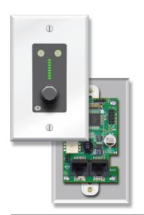
The **ARC-K1e** features a push-button rotary encoder providing simple control of one or two parameters (typically volume) in the Symetrix DSP hardware. An 8-segment LED ladder provides instant user feedback, clearly indicating relative levels. Two additional LEDs illuminate to show which of the two controls is active.
