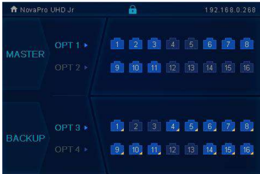
Figure 4-3 Optical fiber port statuses – Hot backup
