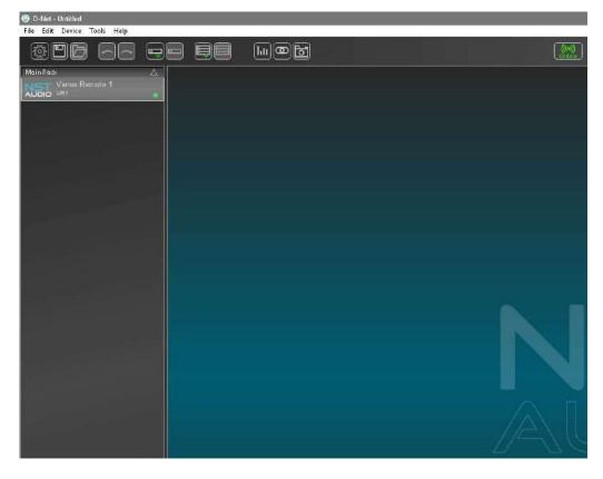
To access the VR1's control panel, simply double click / tap the VR1 device on the left. This will open the VR1's control panel, to allow initial set-up or editing of an existing device.
