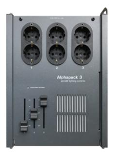
Alphapack 3 range are 3 channel fully portable dimmer units, which can be safely secured to a stand or truss with the use of a hookclamp or half coupler, connected to either of the M10 threaded mounting holes on the top and rear of the unit. Alternatively the optional mounting bracket (sold separately) allows Alphapack 3 to be mounted onto a wall or piece of scenery.
