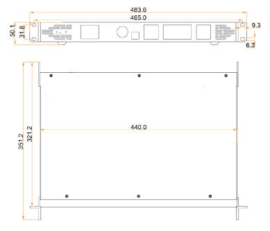
Tolerance: ±0.3 Unit: mm
