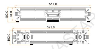
Tolerance: ±5 Unit: mm
