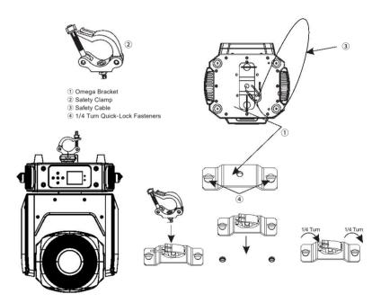
Regardless of the rigging option you choose for your LEDE 20S, always be sure to secure your fixture with a safety cable. The fixture provides a built-in rigging point for a safety cable on the hanging bracket as illustrated above. Be sure to only use the designated rigging point for the safety cable and never secure a safety cable to a carrying handle.
