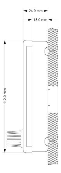
The VR2 wall panel control uses power over ethernet (PoE) to operate. The power requirements are 48VDC, 0.07A with a maximum load of 3.5W. The pin assignment for PoE is shown below:
