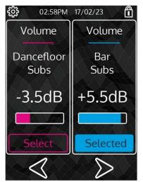
On the VR2, if two gain controls are shown side by side, use the select buttons to decide which one will be adjusted by the rotary.
