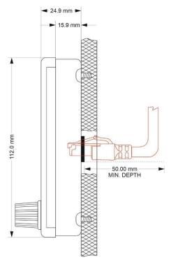
The VR2 will also require a hole in the wall with sufficient size to accommodate the network socket and sufficient depth to accommodate the network cable. Be aware that network cables are variable in their depth requirements – our recommendation is at least 50mm behind the wall surface to ensure that the cable is not bent beyond its specification.
