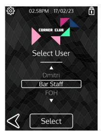
**Set Logo:** The NST Logo shown when the VR2 displays the user list<sup>3</sup> can be changed to match the venue's. The required file format is 24-bit RGB, in png format, with a max resolution of 180W x 60H pixels.
