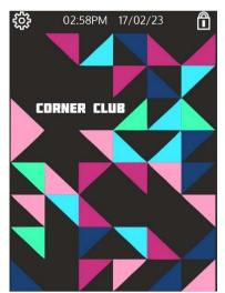
**Set Screensaver:** The NST Logo shown when the VR2 displays the screensaver can be changed to match the venue's. The required file format is 24-bit RGB, in png format, with a max resolution of 320W x 320H pixels.
